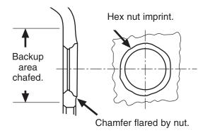
Cause: Loose cap nuts or insufficient preload due to damaged threads or improper torquing or by worn out nuts.
